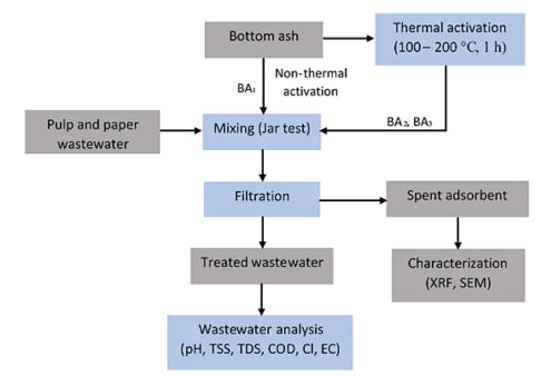
Figure 1. Diagram of pulp and paper wastewater treatment process with bottom ash adsorbent
